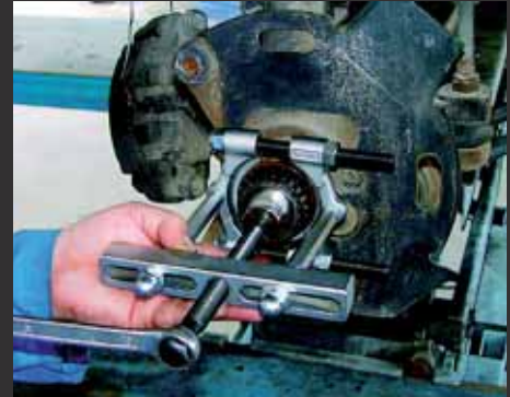
With a special tool, the separator puller, you can safely dismantle two machine parts without damaging them.
