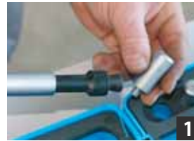
Choose a socket of a suitable size.
