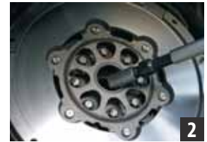
The socket size should suit the flywheel.
