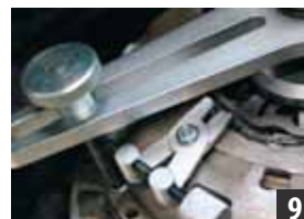
Insert the tool for the tensioning screw.
