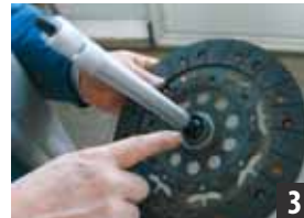
Insert the centering tool into the disc.
