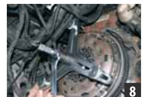
Fasten the tensioner spindle with a suitable wrench.
