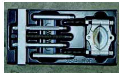
If you turn the gripper assembly of the separator puller, you get a flat bearing surface.
