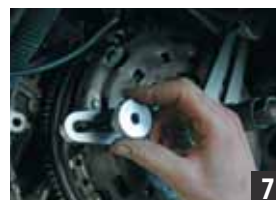
Fasten the nuts onto the tensioner.
