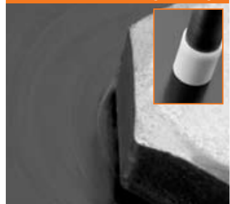
Static covered socket – Light Damage
