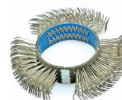
STWW103-23-7 Wire wheel(Coarse) Wire diameter 0.028"(0.7mm) Wheel diameter 4"(103mm) Wheel width 0.91"(23mm)
