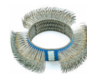
BTWW103-23-5.5 Wire wheel(Medium) Wire diameter 0.019"(0.5mm) Wheel diameter 4"(103mm) Wheel width 0.91"(23mm)
